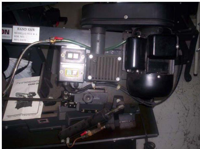
BAND SAW, the run and start capacitors are housed left on the side of the motor.
