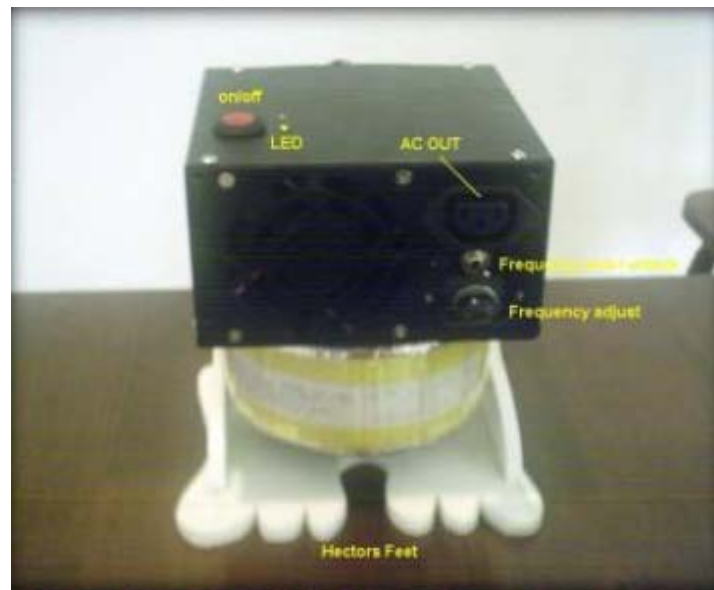
Frequency adjustable inverter built by Phil Wood.
