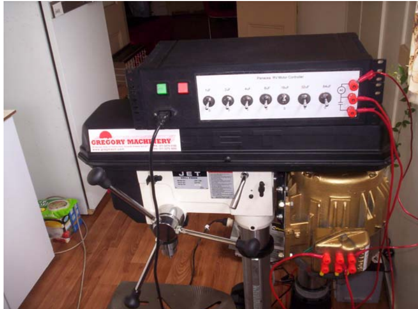
RV Drill press with binary switched Capacitor bank above
