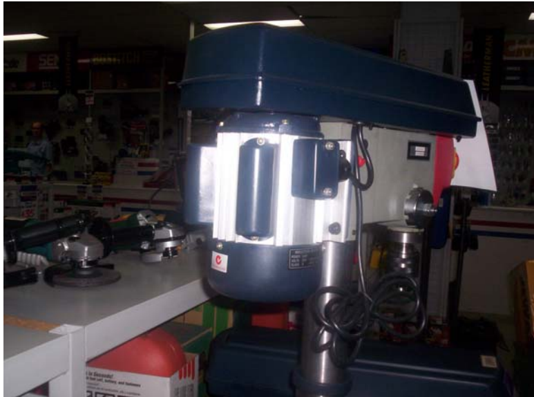
DRILL PRESS, with run and start caps attached left and right side of the motor.
