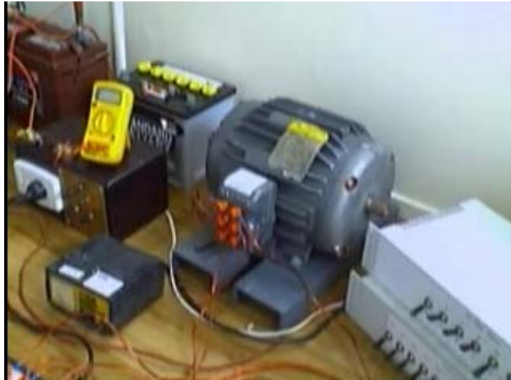
A 5 HP Baldors motor modified to run in RV mode to give .8- 1.13 HP for energy saving applications.
