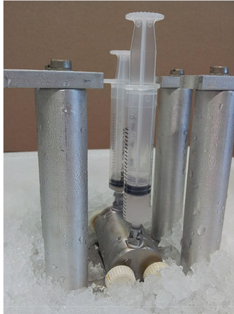
Fig. 3 Balch homogenizer. To keep the homogenate at 4 °C, precool the homogenizer for 15 min on ice. Depending of the volume of PNS use a suitable syringe size (from 1 to 10 ml). The volume of the PNS to be homogenized should not exceed half of the maximum volume of the syringe [16]
