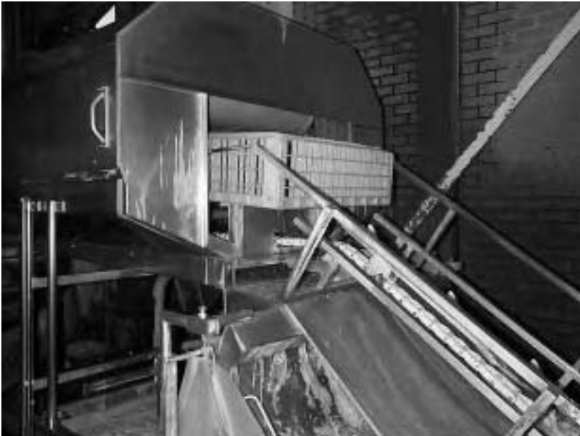
Fig. 6.5 Drawers entering main wash booth. The run-down screen is visible in the lower part of the photograph; some fouling is evident.
