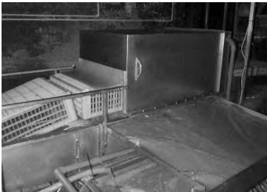
Fig. 6.3 Pre-wash booth and associated water recirculation equipment. The run-down screen that filters the water is just out of view at the bottom right of the photograph. Screened water collects in the main tank, from where it is recycled to the jets in the booth and to the soak tank. Make-up water is added to this tank.
