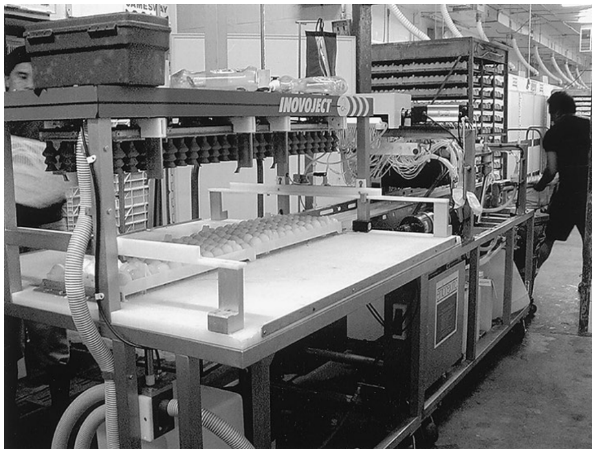
Figure 1.9 A modern hatchery with an egg injection system for in ovo vaccination.
