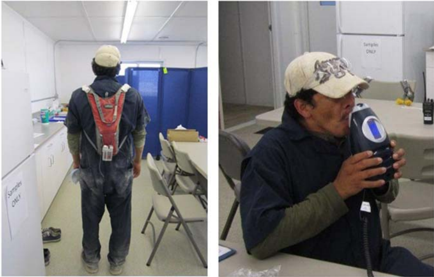
Figure 10.6 One of the most serious health hazards for workers in egg production systems is inhalation of airborne contaminants like dust, ammonia, and endotoxin. Exposure to these contaminants can be assessed by asking them to wear a backpack throughout the workday like the one shown, which has air samplers located on the shoulders to measure particulate matter and ammonia exposure. Lung function after a work shift can then be tested using spirometry. For details see Arteaga et al. (2015) and Mitchell et al. (2015) .
