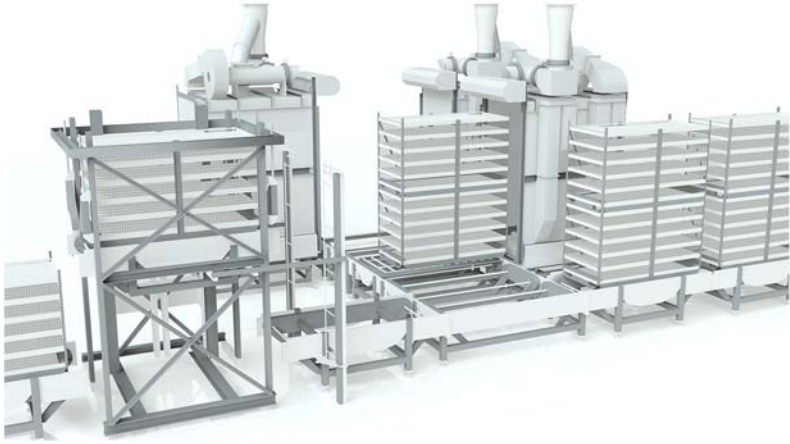
Figure 5.3 Single transport unit turkey controlled atmosphere stunning (CAS) unit that allows for both an irreversible and reversible stun of the birds.
