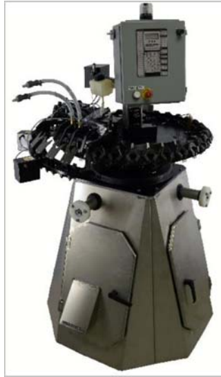
Figure 2.2 Nova-Tech Poultry Service Processor (PSP) equipment used for infrared beak treatment (IRBT). Chicks are placed on this equipment after hatch, where the tip of the beak is exposed to an infrared light. Vaccination also takes place on the same equipment, reducing the need for manual handling of chicks.
