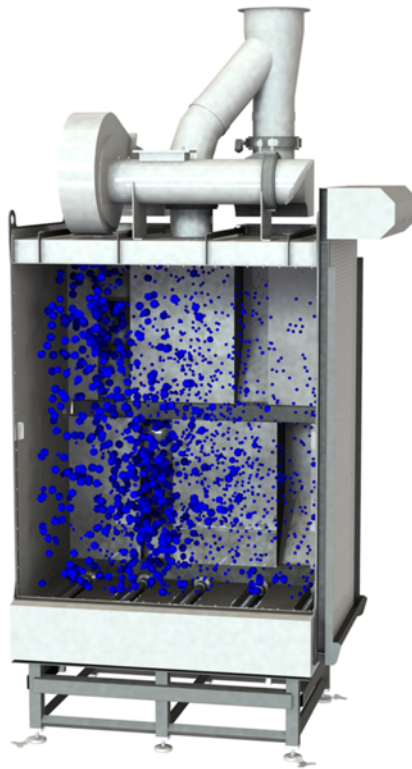
Figure 5.1 (A) Controlled atmosphere stunning (CAS) system that moves birds in transport container through various levels of gas. The closed cabinet construction allows for the carbon dioxide concentration to be precisely controlled in every stage of the process, ensuring a humane stun and improved product quality. (B) Airflow in vertical multistage CO 2 system.
