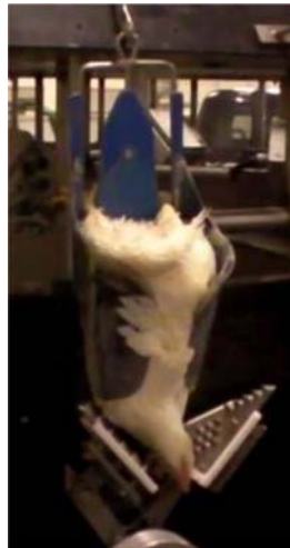
Figure 4.5 Head-only electrical stunning. The broiler is restrained in a cone with open electrode plates just before stunning.
