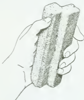
Prismatic sandstone from Missouri. The prisms are about an inch wide. (X1)
